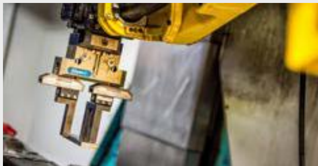
Part picking by robot
