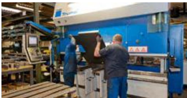
Computer assisted steel plate bending
