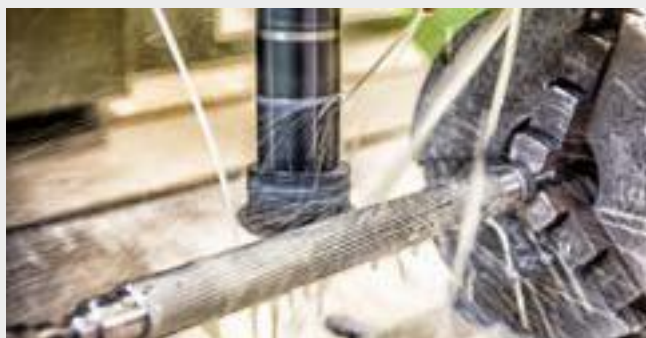
Milling of drive roll
