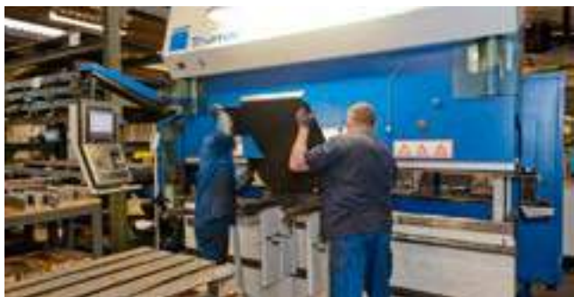
Computer assisted steel plate bending
