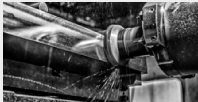
Edge milling of cast iron table
