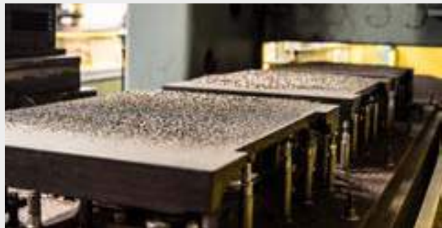
Surface scraping of cast iron table
